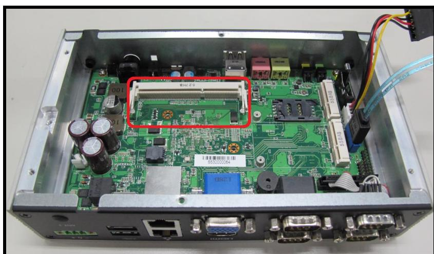
**Step 5** Locate the memory module, insert the gold colored of memory to contact into the socket.
