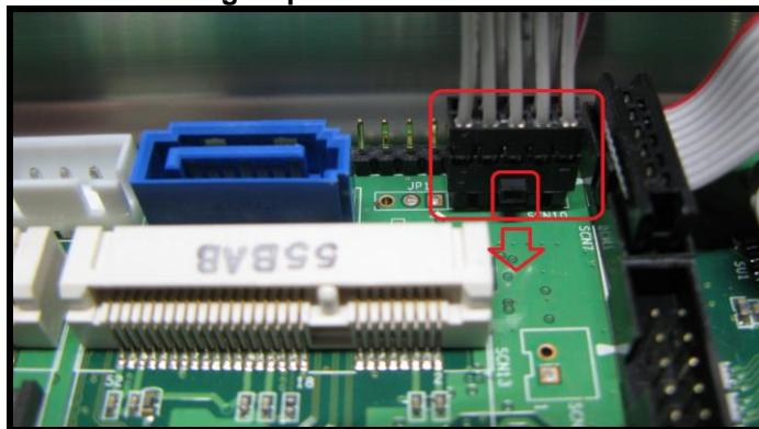
**Step 6** Fasten two hexagon pillars with 8-CH DIO connector then complete installation.
