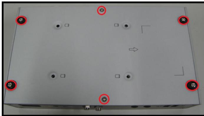
**Step 3** Remove the bottom cover and then prepare your 2.5" HDD/SSD to assemble with your bottom cover.
