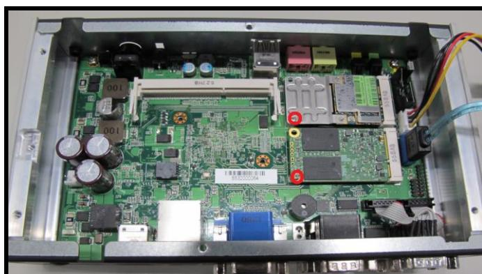
**Step 5 Assembly the bottom cover back and fasten all screws to finish installation.**
