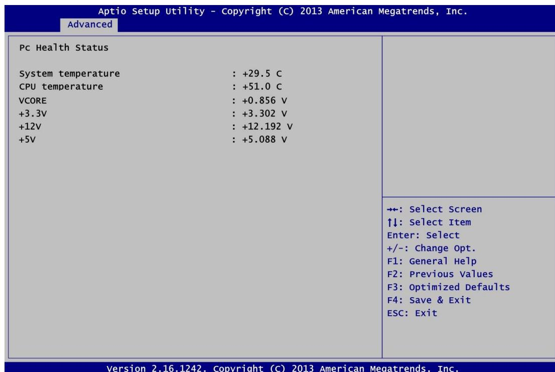
This screen displays the temperature of system and CPU, and system voltages (VCORE, +3.3V, +12V and +5V).
