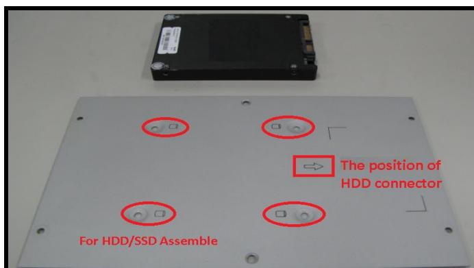
**Step 5** Assembly the HDD on bottom cover and notice the connector position.
