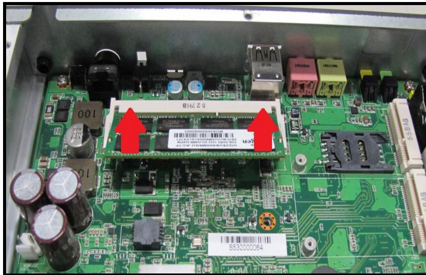
**Step 6** Push the module down, until it is firmly seated by locking two latches on the sides.
